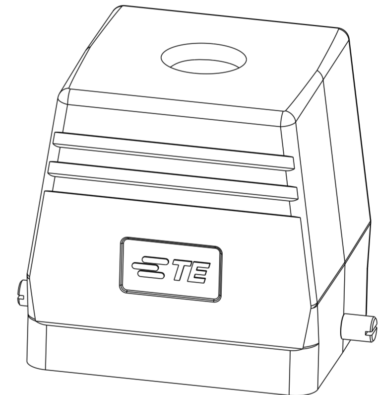
TYPE 5: HIGH CONSTRUCTION, TOP ENTRY, UNDEFINED DIMENSIONS REFER TO TYPE 4. 类型5: 高结构, 顶出, 未定义尺寸 & 规格参照类型4.
