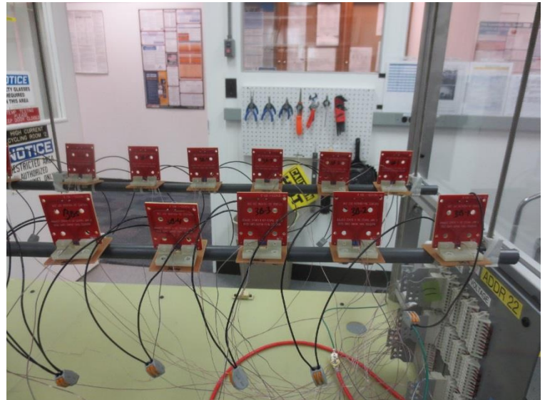
Figure 2 Temperature Rise Set Up
