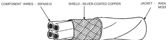
RADIATION-CROSSLINKED, MODIFIED CONDUCTIVE ETFE
