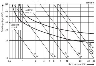
Load limit curve 1: arc extinguishes during transit time (CO contact). Load limit curve 2: safe shutdown, no stationary arc (NO contact). Load limit curves measured with low inductive resistors verified for 1000 switching events.
