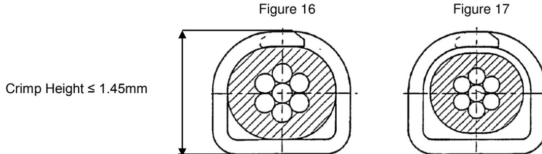
Contacts as well as housing shall show no signs of damage or deformation due to the wire termination process.
