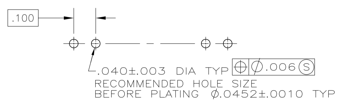
RECOMMENDED HOLE LAYOUT
