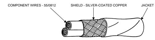
JACKET - LOW OUTGASSING, RADIATION-CROSSLINKED, MODIFIED ETFE
