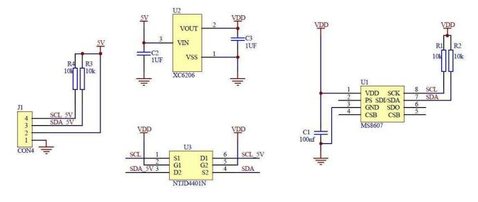
Connector Pin Assignments (I<sup>2</sup>C Communications)
