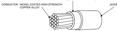
JACKET - RADIATION-CROSSLINKED, MODIFIED ETFE
