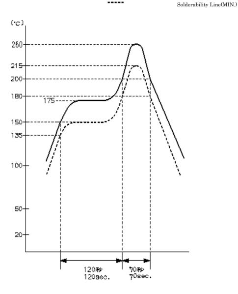
Fig. 3 Reflow Condition
