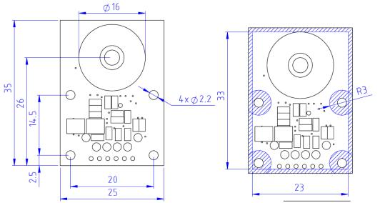
Only use hatched areas for mechanical assembly (screws, nuts, etc).
