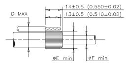
The cable shield should be folded back over the jacket and trimmed to the length as shown.
