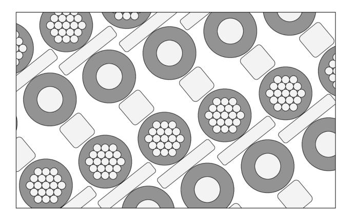
For best results, the proper terminal or splice must be selected not by the "fit" of wire or wires in the terminal barrel, but by the total circular mil area in cross section of the wires used. For this purpose convenient tables have been prepared to assist in the calculation of circular mil areas. When the totals are known, the proper terminal or splice can be determined quickly.
