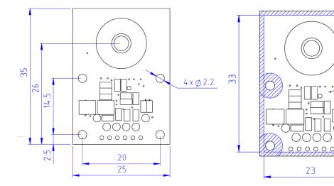
Only use hatched areas for mechanical assembly (screws, nuts,
