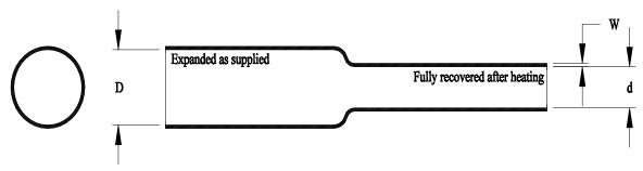
This specification covers the requirements for one type of single wall, electrical insulating, extruded tubing whose diameter will reduce to a predetermined size upon application of heat in excess of  $140^{\circ}$ C (284°F).
