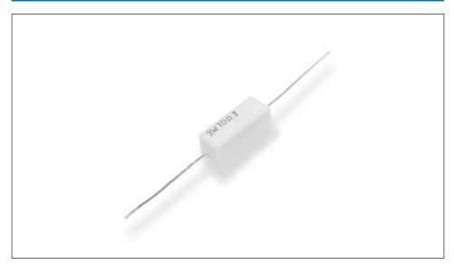
There are some similarities between resistors and fuses in material and structure. Fusible Resistors contain both functions, as a resistor in normal conditions and as a fuse when abnormal currents are applied, so to protect machinery and equipment. Cost savings are apparent as one component is eliminated. The FSQ Fusible Resistor series are produced with precision techniques, enabling precise and stable fusing times.
