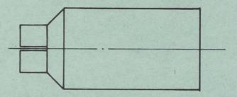
Provides a larger volume of heated air at a lower temperature than is obtained with no tip. Used to install heat-shrinkable molded parts and tubing without hot-spot overheating.
