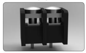
The captive clamp is designed to accept multiple wires and wire gauges. With the captive clamp, you save time! No need to loop the wire, you just strip & screw down underneath the clamp. The clamp rides up and down with the screw.
