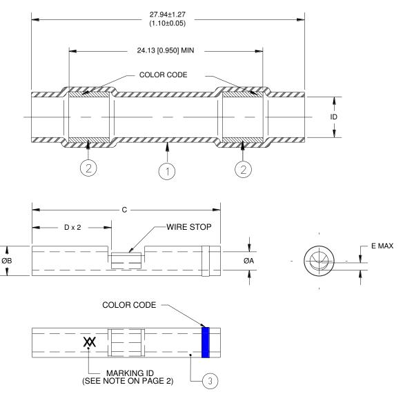
\* I.D.: a) As received; b) After unrestricted recovery thru meltable insert.
