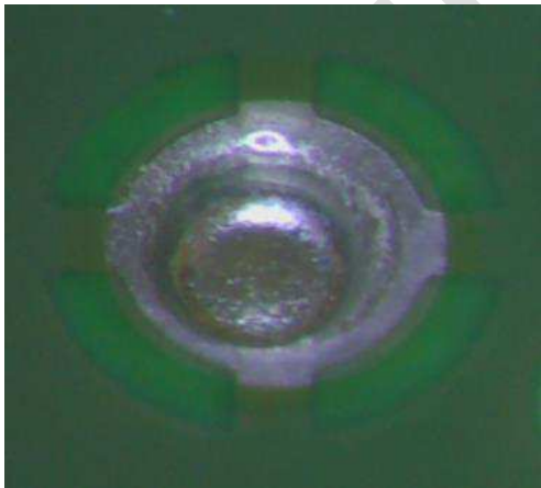
Soldered ground pin Lötstelle Masse-Pin
