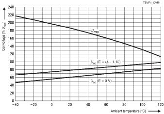
Does not take into account the temperature rise due to the contact current F = pre-energization
