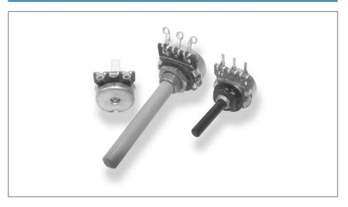
TE Connectivity will customize these neat 16mm diameter control potentiometers to suit your requirements. They comprise a printed carbon resistance element with 0.25 W current handling and are available with various bush, termination and spindle styles.
