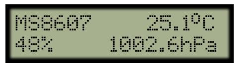
Sensor measurements are refreshed every 500 milliseconds.
