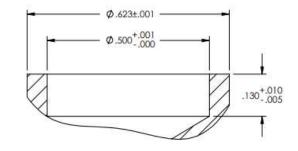
NOTE: WELD WELD PREP SHOWN IS FOR RESISTANCE WELD, ACTUAL GEOMETERY VARIES PER CUSTOMER REQUIREMENTS
