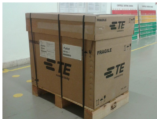
Fig. 1: Proper packing of relays for transportation
