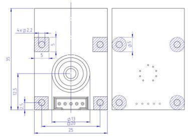
Only use hatched areas for mechanical assembly (screws, nuts, etc).
