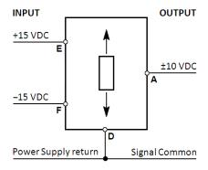
A through F: Connector pin assignments
