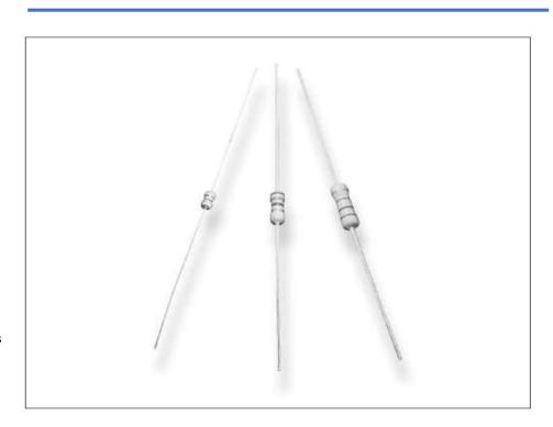
The resistive element comprises a thin film of carbon, deposited onto a high thermal conductivity ceramic core. Metal end caps are force fitted to the element prior to spiralling to value. Tinned copper lead wires are welded to the end caps and the components are then coated. One coat of phenolic resin is followed by three coats of epoxy resin. All resistors are tested for value and tolerance.
