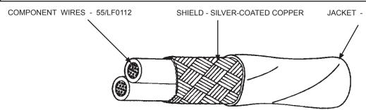
JACKET - LOW OUTGASSING, ULTRA LOW FLUORIDE, RADIATION-CROSSLINKED, MODIFIED ETFE
