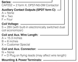
D = 2X M5 Bottom Mount with 4X, M6 x 1 Female thread terminals
