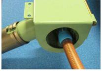
o. Apply heat to the Solder Sleeve until the solder melts and the heat shrink tubing recovers. SolderSleeve is recovered when the solder ring has fully melted and the blue thermoplastic seals melt and seep past the edge of the sleeve. Note that slight flux residue may be visible after the solder melts.
