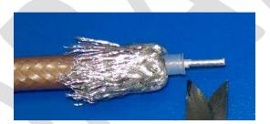
Place the SolderSleeve onto the left cable end, with the small opening to the left.
