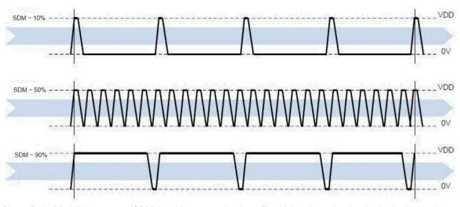
Sigma Delta Modulation output (SDM) is a bit-stream of pulses. The higher the pulse density is, the higher the measured temperature. The fundamental frequency of SDM is in the range of roughly  $4\,\mathrm{kHz}$  and  $65\,\mathrm{kHz}$
