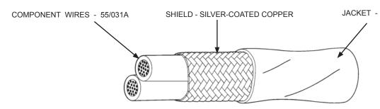
JACKET - LOW OUTGASSING, RADIATION-CROSSLINKED, MODIFIED ETFE
