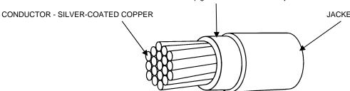
JACKET - RADIATION-CROSSLINKED, MODIFIED ETFE
