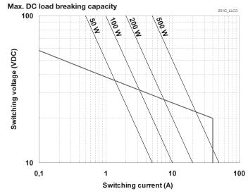
Load limit curve: safe shutdown, no stationary arc/make contact. Load limit curves measured with low inductive resistors verified for 1000 switching events.
