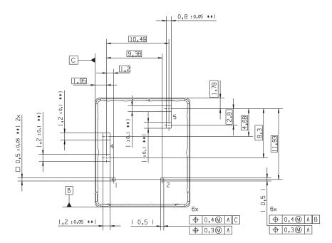
Remark: Positional tolerances according to DIN EN ISO 5458 \*\*) without tinning (hot dip)
