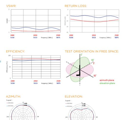
DATA AND DEVICES /// 2400-2500 & 5150-5875 MHz DUAL BAND ANTENNA
