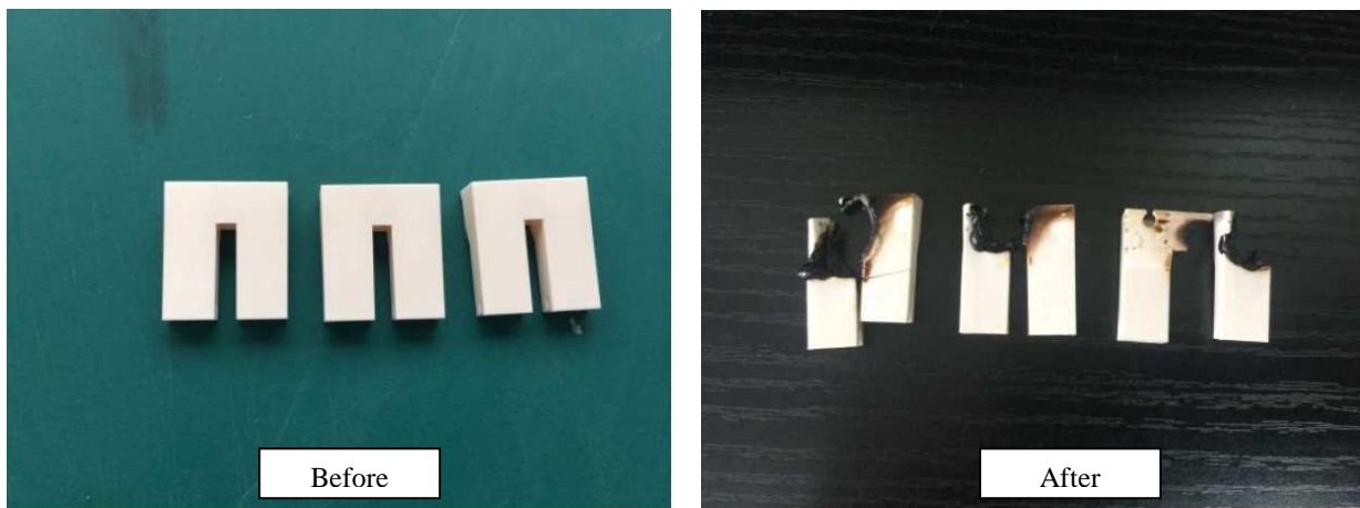
Figure 3 – visual check for GWT 750°C test
