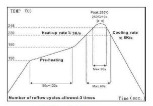
IR Reflow Soldering (1) Time of IR reflow soldering at maximum temperature point 260°C : 10s
