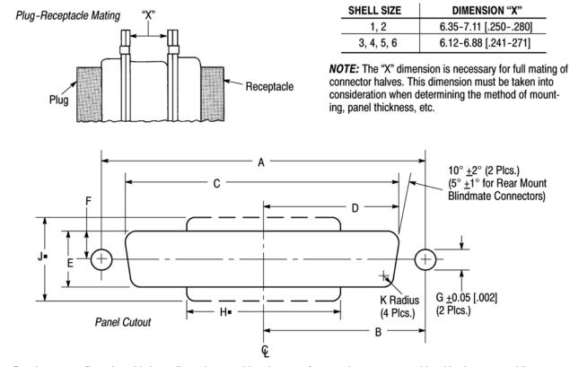
Panel cutout configuration with these dimensions provides clearance for mounting connectors with cable clamp assemblies. **NOTE:** When front mounting a MIL-DTL-24308 connector utilizing the tab method of securing shell halves, it is recommended to utilize a 0.81 [.032] thick washer (not supplied) to prevent deformation of the connector flange.
