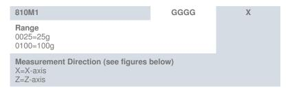
Examples; 810M1-0025X Model 810M1, 25g range, X-axis measurement
