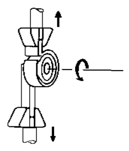
FIGURE 1 Peel test specimen in Tensile Tester
