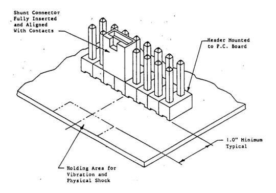
Figure 4 Vibration and Physical Shock
