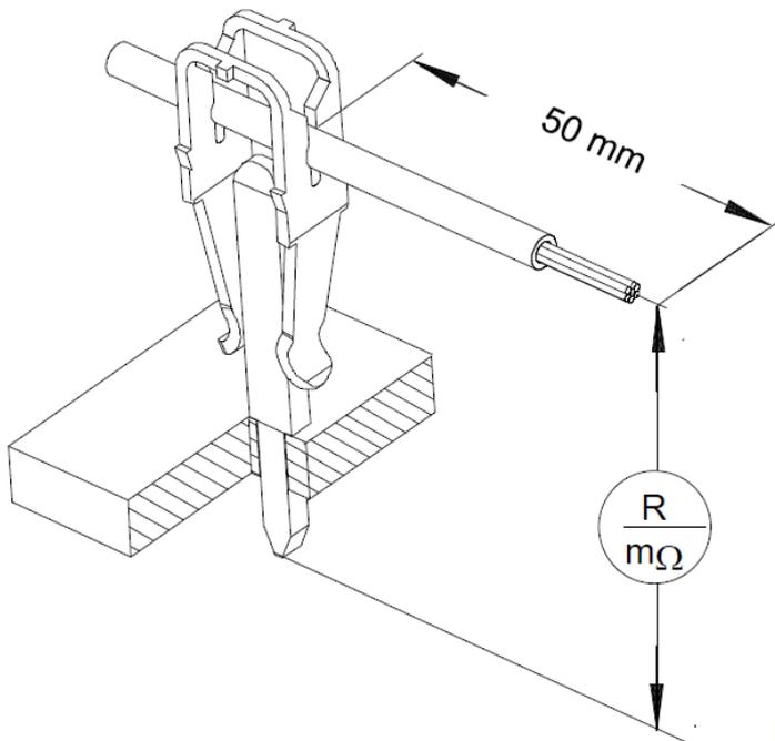
$$R_g = R - R_{50\text{mm Draht}}$$
