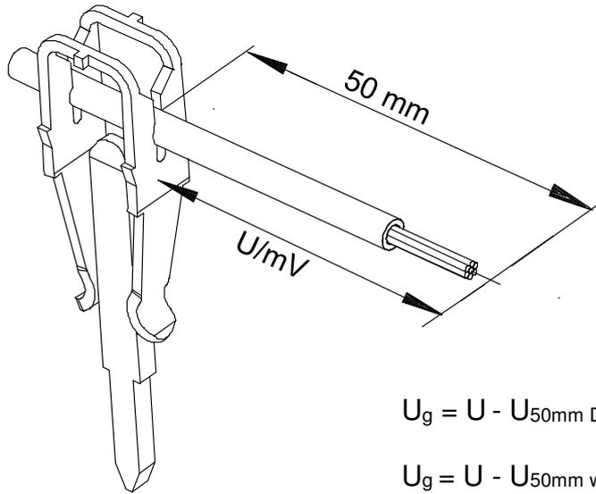
$$U_g = U - U_{50\text{mm Draht}}$$
