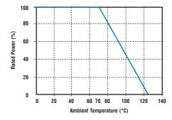
When the ambient temperature exceeds 70°C, reduce the rated power and current in accordance with the derating curve shown
