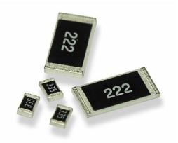
The resistive element is screen printed and fired, and a passivation layer added. Each resistor is trimmed to tolerance by laser. The pre-scribed tile is then broken into strips, the end plating fired on, and the strips broken into individual components. Final termination finish is electroplated matte Sn over a Ni barrier layer.
