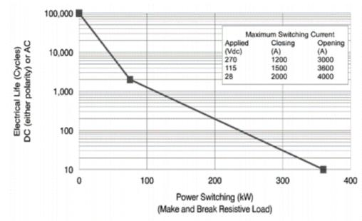
\*Failure Mode: Dielectric withstand voltage test @ 2000 Vdc, power terminal to terminal, leakage exceeds 1.0 mA. Current carry: 500 A @ 25°C. Derate 2.5 A/°C to 350 A @ 85°C for still air, no heat sink, AWG# 00 conductor.
