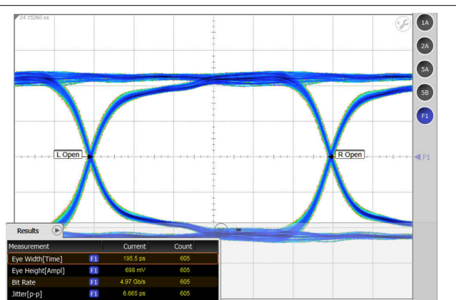
Figure 9-4. 5 Gbps PRBS-7 Signals Through a Typical TMUXHS4212 Channel in TI Evaluation Board
