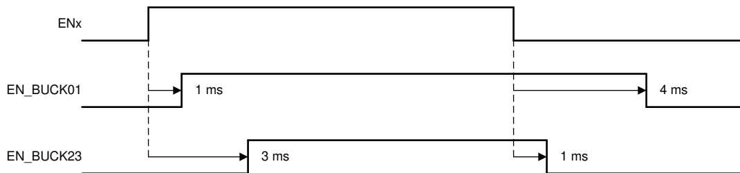
Figure 16. Typical Start-Up and Shutdown Sequencing
