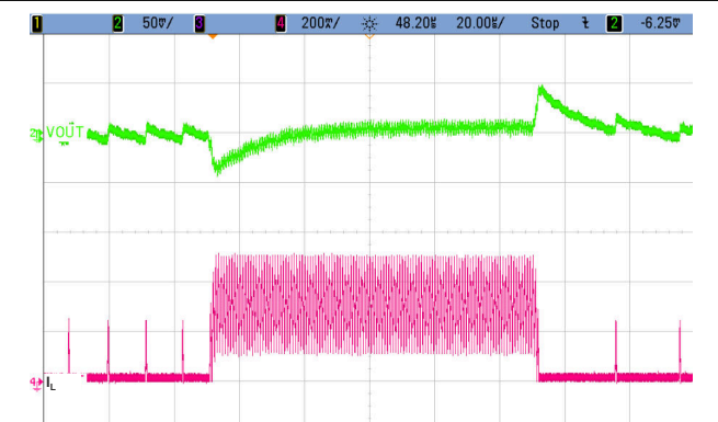
Figure 9-20. Load Transient Response; 5 mA to 290 mA
