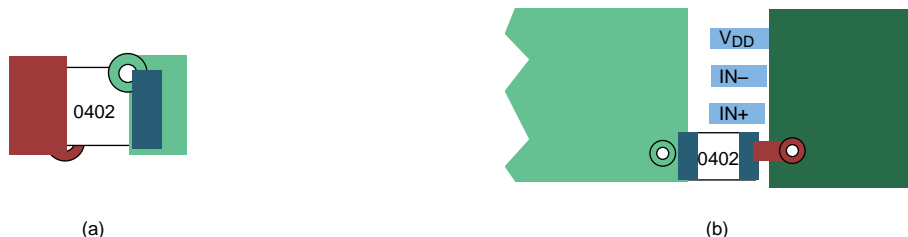
Figure 33. Typical Decoupling Capacitor Layouts
